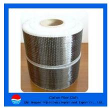
1.Introduction: Carbon fiber cloth is pressed with carbon fiber and resin, which is used for tensile, shear and seismic reinforcement of structural components. The product and matching impregnating adhesive are used together to form carbon fiber composite material, which can form a complete and excellent carbon fiber cloth sheet reinforcement system, suitable for protection and reinforcement of building engineering, structural crack treatment, material aging
