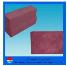
1.Introduction: using  $\alpha$  - Al2O3 as raw material, adding chrome oxide powder or chrome corundum clinker powder, forming by high-pressure molding machine or vibration molding machine, firing in high-temperature shuttle kiln at 1600 °C ~ 1700 °C. Because the product has good high temperature performance and is used at 1700 °C, it is widely used in various high temperature resistant, corrosion-resistant and wear-resistant furnace equipment.
